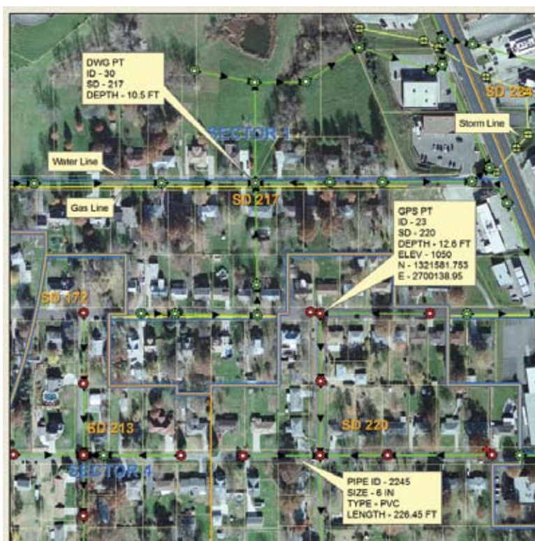
This image demonstrates the city of St. Joseph's sanitary sewer network and associated attributes within their GIS mapping program.
